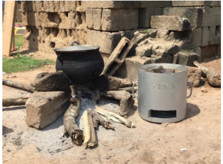
Typical "3 Stone" fire and the Tika cookstove
